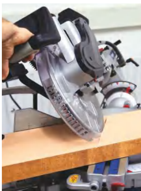
▲ Pic.17 The smallest of fixed woodworking machines such as this sliding cross-cut saw are handy for cutting angles or straight ends on relatively narrow pieces of wood
